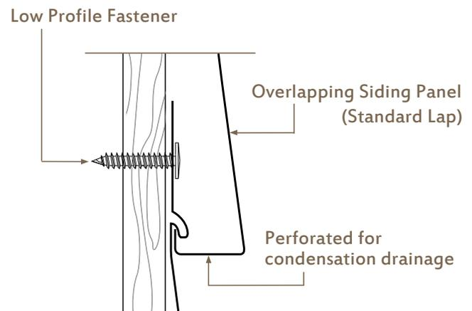
Fasten Panel to Wood with #10-9 Low Profile Wood Screw
